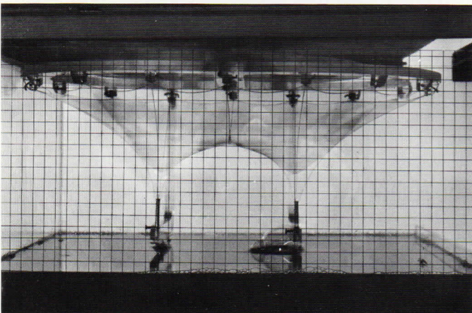
Soap films illustrate "minimal principles." The machine above enables designers to determine the surface area and stresses in the structure produced by inverting the soap film (upper right). The soap-film-inspired
